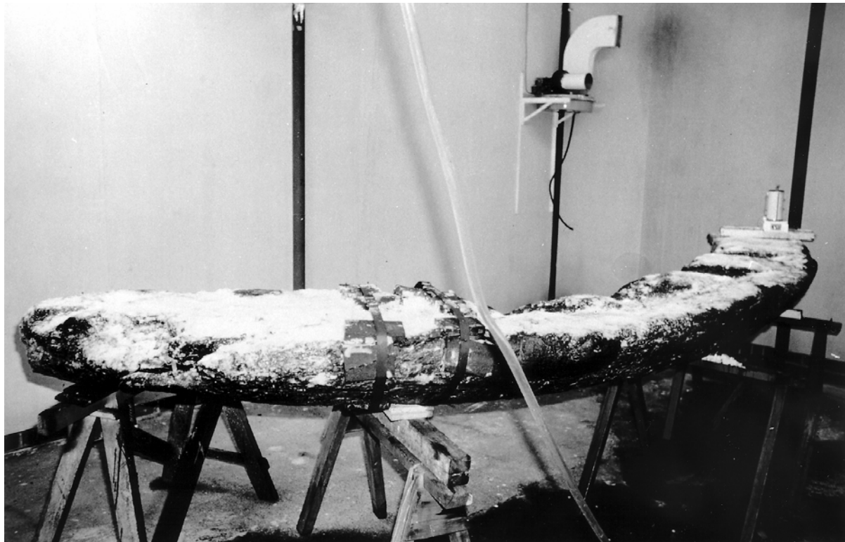
Figure 2. Second generation dehumidification chambers with the fashion piece undergoing drying. Photo: Jon Carpenter.
